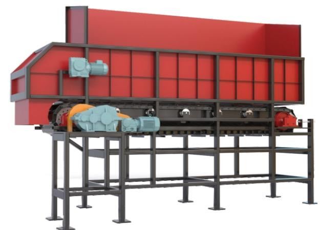
Suitable for short distance transportation from storage bin to crusher, shaker, batching and other mechanical equipment. Uniform feeding, no manual operation, with its own pulling function,board chain feeder has greater adaptability to the material,not limited by the size of the material,specific gravity.
